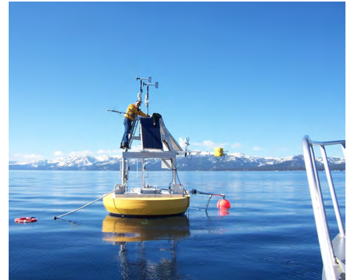
Brant Allen changes out an atmospheric bucket from one of four NASA buoys that were all installed and transported by the R/V LeConte . (Brandon Berry, UC Davis TERC)
