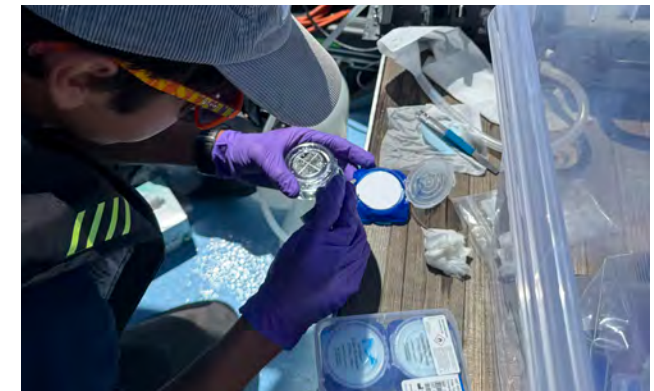
Dante Capone uses fragile, specialized filters to collect DNA from lake samples to study the lake's microbiome. Collecting data while the air is clear will establish baseline data to better understand future wildfire smoke impacts. (Cara Hollis, UC Davis TERC)
