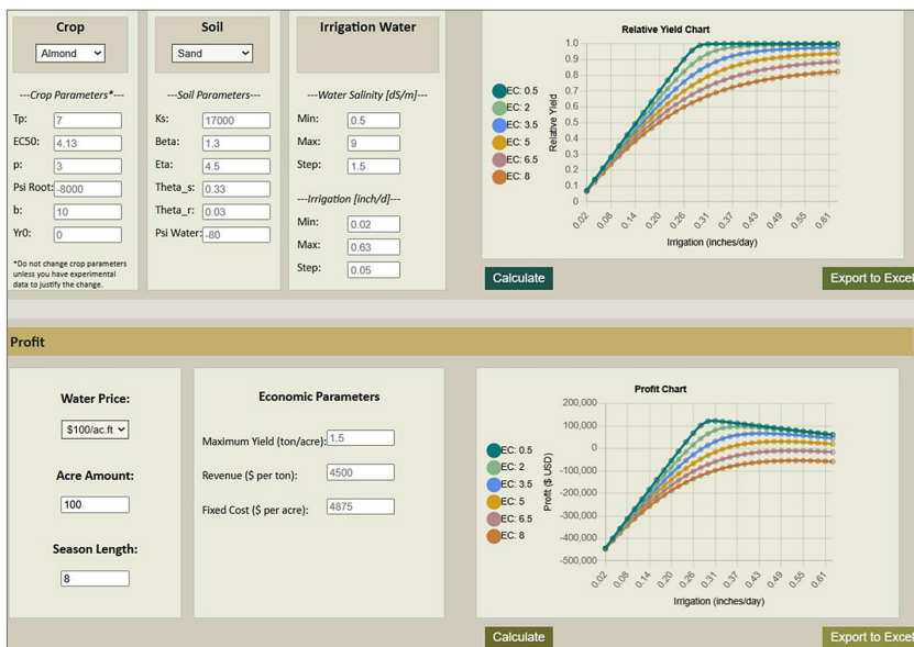
FIG. 3. Web tool yield and profits calculation interface (example scenario). The upper panel collects agronomic inputs to calculate and plot relative yield for each EC_{iw} level. The lower panel uses economic inputs to compute and plot profits with irrigation amount and EC_{iw} levels.
