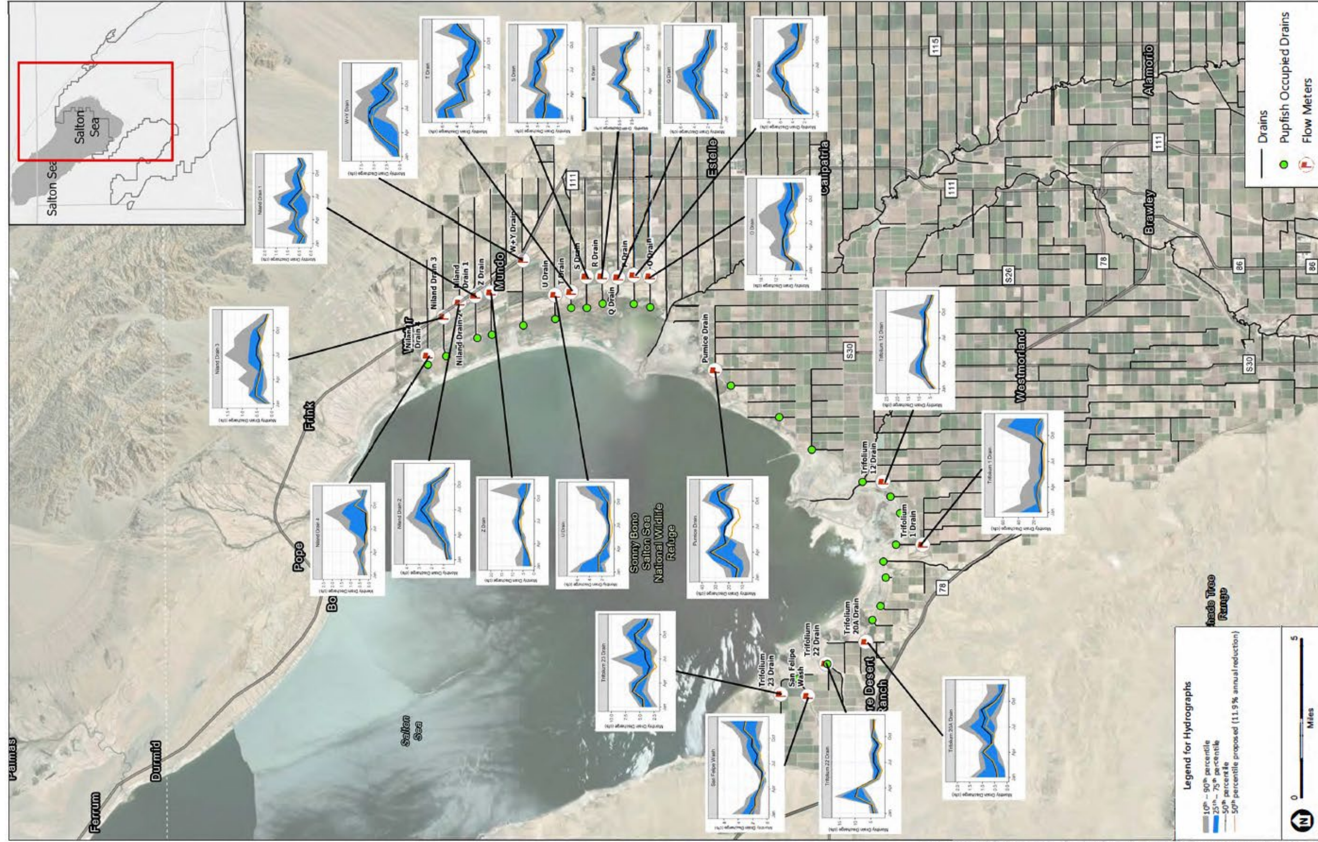
Figure 3-5 Drain Flow Hydrographs
