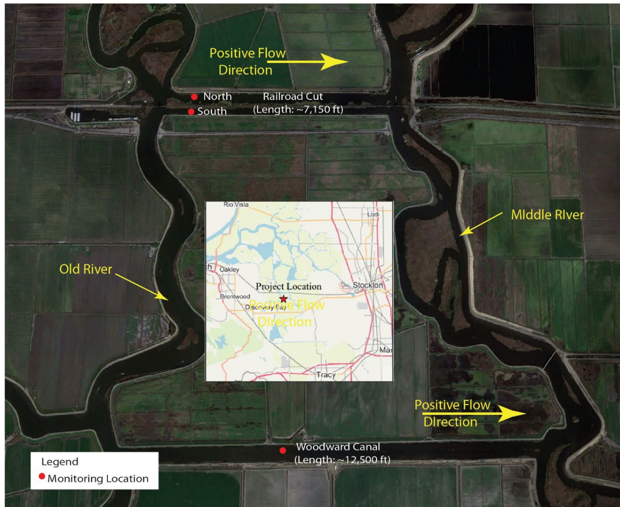
Figure 2.2.2-35 Locations of Railroad Cut and Woodward Canal flow and salinity monitoring stations in the Sacramento–San Joaquin Delta.
