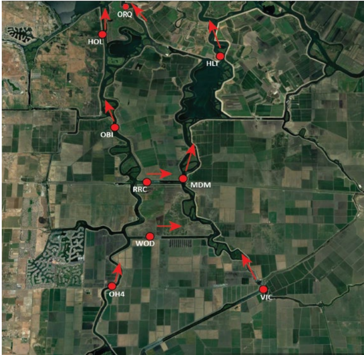
Figure 2.2.2-36 Direction of positive (ebb) flow across various DWR and U.S. Geological Survey monitoring stations.
